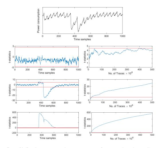
**Figure 14:** Sample power trace and univariate non-specific *t*-test results with 500 million measurements for two composed DOM-*indep* multiplications (d = 2) based on  $GF(2^4)$  multipliers without output registers but with pipeline registers applied. The second to fourth row show the *t*-statistics for the statistical moments 1 to 3, respectively.
