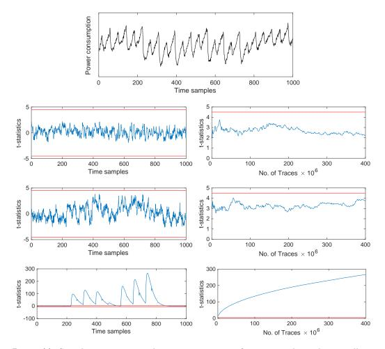
**Figure 11:** Sample power trace and univariate non-specific *t*-test results with 400 million measurements for two composed UMA multiplications with d = 2, based on  $GF(2^4)$  multipliers. The second to fourth rows show the *t*-statistics for the statistical moments 1 to 3, respectively, arranged like before.
