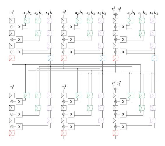
**Figure 10:** Composition of two UMA multiplications (d = 2) with several kinds of (mandatory and optional) pipelining and synchronization register stages.
