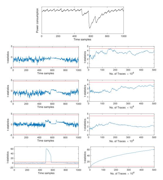
**Figure 8:** Sample power trace and univariate non-specific *t*-test results with 500 million measurements for a single DOM-*dep* multiplier with d = 3, based on  $GF(2^4)$  multiplications. The second to fifth rows show the *t*-statistics for statistical moments 1 to 4.
