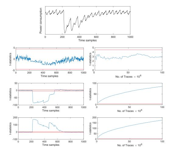
**Figure 20:** Sample power trace and univariate non-specific *t*-test results with 100 million measurements for two composed UMA multiplications (d = 2) based on  $GF(2^4)$  multipliers with only the mandatory registers applied. The second to fourth row show the *t*-statistics for the statistical moments 1 to 3, respectively, arranged like before.
