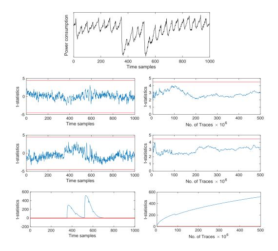
**Figure 16:** Sample power trace and univariate non-specific *t*-test results with 500 million measurements for two composed DOM-indep multiplications (d = 2) based on  $GF(2^4)$  multipliers with all registers applied. The second to fourth row show the *t*-statistics for the statistical moments 1 to 3, respectively, arranged like before.
