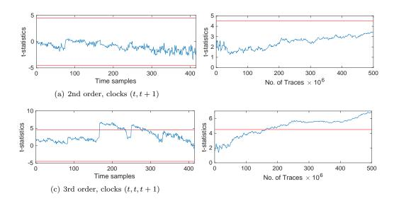
**Figure 9:** Multivariate non-specific *t*-test results with 500 million measurements for a single DOM-*dep* multiplier with d = 3, based on  $GF(2^4)$  multiplications.
