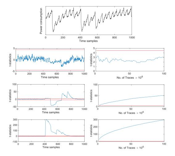
**Figure 19:** Sample power trace and univariate non-specific *t*-test results with 100 million measurements for two composed DOM-*indep* multiplications (d = 2) based on  $GF(2^4)$  multipliers with output registers but without pipeline registers applied. The second to fourth row show the *t*-statistics for the statistical moments 1 to 3.
