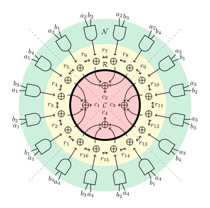
**Figure 1:** Architecture of CMS multiplication extending the proposal in [CRB<sup>+</sup>16] to d = 3, consisting of the (green) non-linear layer  $\mathcal{N}$ , the (yellow) (ring) refresh layer  $\mathcal{R}$ , the (black) synchronization (registers) layer  $\mathcal{S}$ , and the (red) compression layer  $\mathcal{C}$ .
