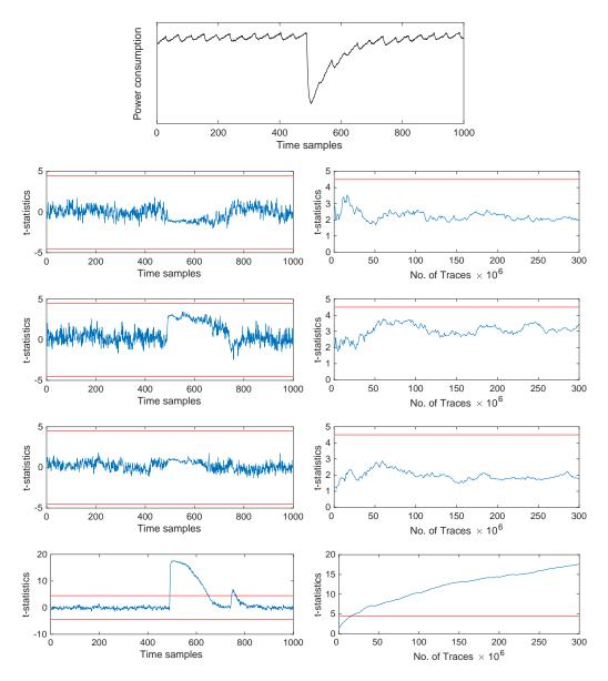
**Figure 6:** Sample power trace and univariate non-specific *t*-test results with 300 million measurements for a single  $GF(2^4)$  multiplier masked by means of CMS with d = 3. The second to fifth rows show the *t*-statistics for the statistical moments 1 to 4, respectively. The left column depicts the *t*-values over time, the right column illustrates the evolution of the absolute maximum *t*-value over the number of traces.
