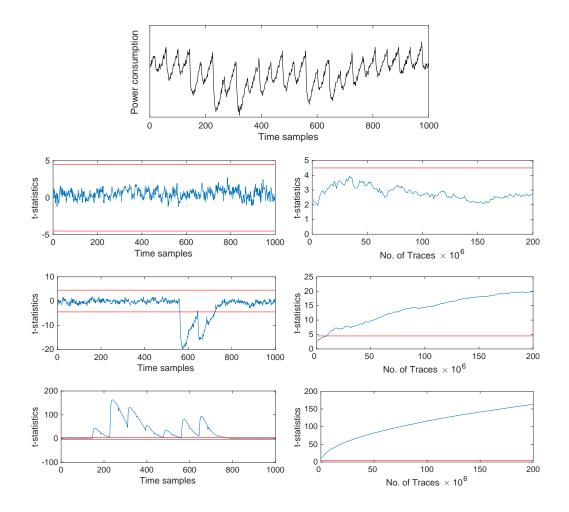
**Figure 18:** Sample power trace and univariate non-specific *t*-test results with 200 million measurements for two composed UMA multiplications (d = 2) based on  $GF(2^4)$  multipliers without pipeline registers for the inner-domain terms. The second to fourth row show the *t*-statistics for the statistical moments 1 to 3, respectively.
