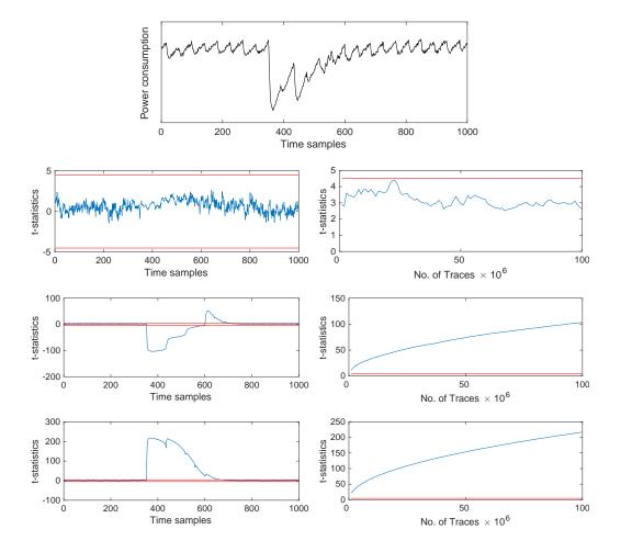
**Figure 21:** Sample power trace and univariate non-specific *t*-test results with 100 million measurements for two composed DOM-*indep* multiplications (d = 2) based on  $GF(2^4)$  multipliers with only the mandatory registers applied. The second to fourth row show the *t*-statistics for the statistical moments 1 to 3, respectively, arranged like before.
