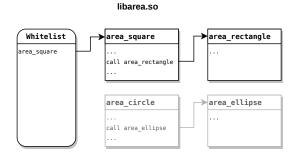
Fig. 2: Example of the basic idea of the analysis. A target application uses the function <code>area\_square</code>. Hence, the function <code>area\_rectangle</code> is also added to the whitelist.
