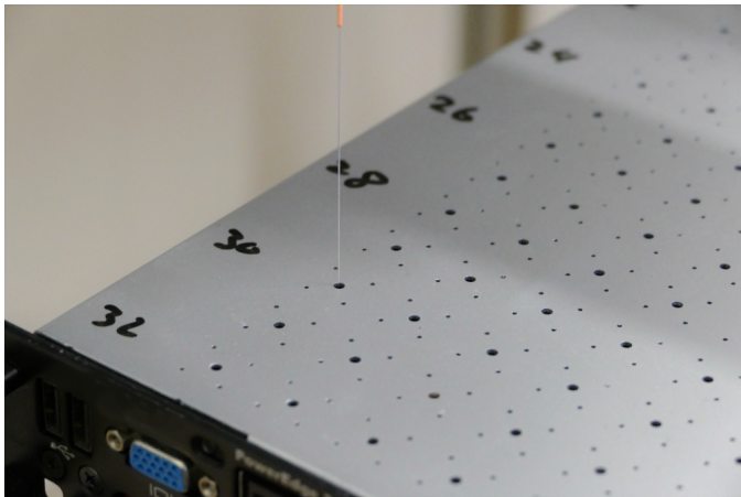
Fig. 6. Close view of the server lid with drills and probing needle.
